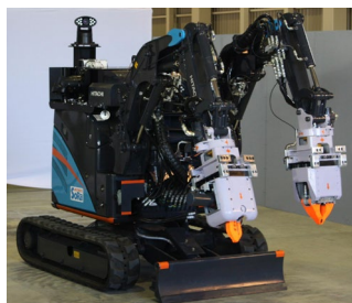
Debris removal robot - remote control work
