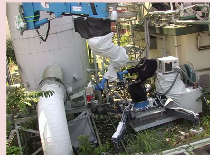
Collaborative operation of crawler/crane robots
