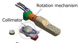
Gamma camera Development of radiation measurement device with gamma camera
